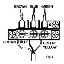
If the cable has to be threaded through small apertures in cabinets etc., it may be disconnected from the appliance, then re-connected to as shown in Fig.4.
